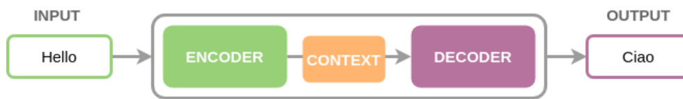
Figure 3: The architecture of an encoder-decoder (or sequence-to-sequence) model
