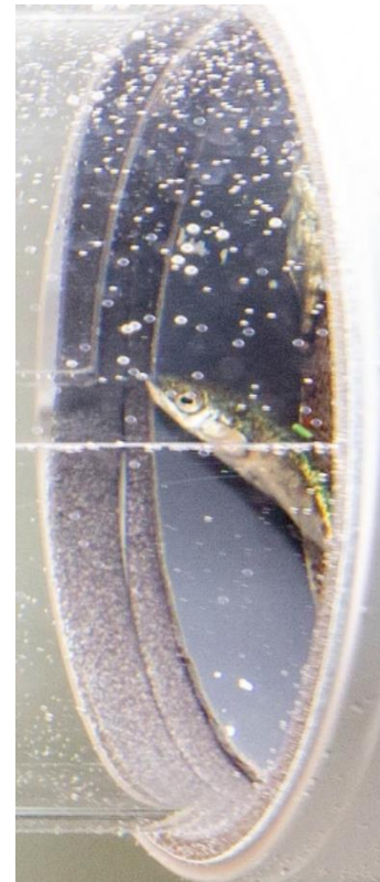
Figure 12: Fish being pushed against the grid by the flow.
