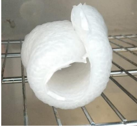
Figure 11. Ecoflex + ethanol and paper actuator fully bent during heat application
