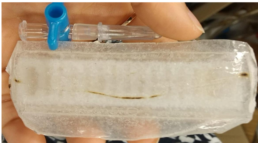
Figure 1. Device manufacturing attempt using a straight stainless-steel wire
