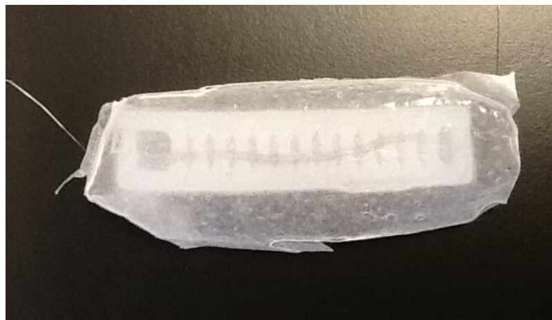
Figure 5. Device enclosed by cellulosic paper and Sylgard 184 PDMS
