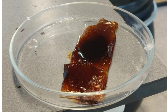
Figure 10. Spin coated bilayer composed of polyketone on the bottom and Sylgard 184 PDMS on top glued over a glass substrate
