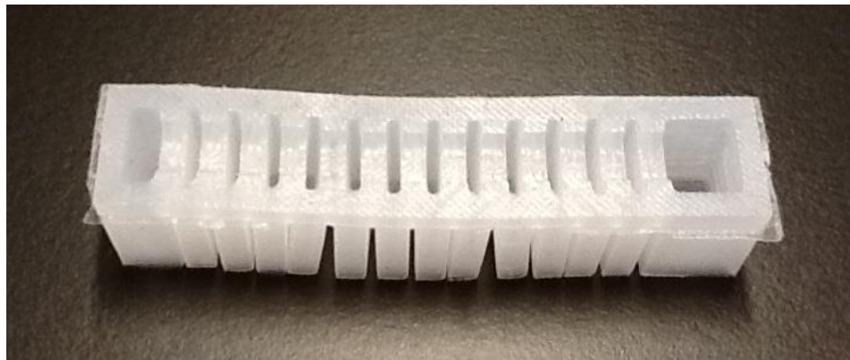
Figure 4. Hollow device before closing made out of Ecoflex 00-50
