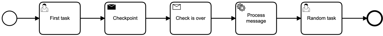
Figure 6: BPMN representation of the adaptable process model from Figure 5. We can note the “checkpoint send task” labelled as Checkpoint , the “message receive task” labelled as Check is over and the “message processing service task” labelled as Process message , all three of which make up the “checkpoint state”.
