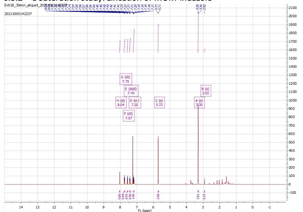
Figure 74: ^1\text{H-NMR} spectrum of deuterated MOM-indazole using \text{TMP}_2\text{Zn} in \text{CDCl}_3 . Bar from a few impurities, it is clear is this MOM-indazole with mediocre metalation at best.
