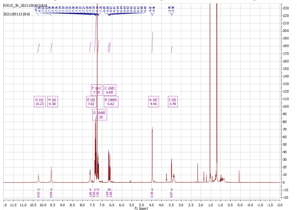
Figure 59: ^1\text{H-NMR} spectrum of the 3 h aliquot of the reaction mixture in \text{CDCl}_3 . Note the NH signal around 9.6 and 10.4 ppm.
