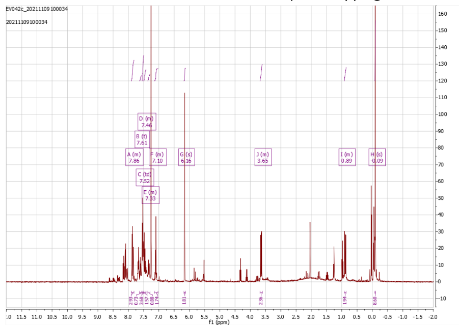
Figure 92: ^1\text{H-NMR} spectrum crude 24 in \text{CDCl}_3 . The regions that are analysed are based on what was reported in literature. The integrations are higher than reported in the aromatic region due to significant signal overlap with side product signals.
