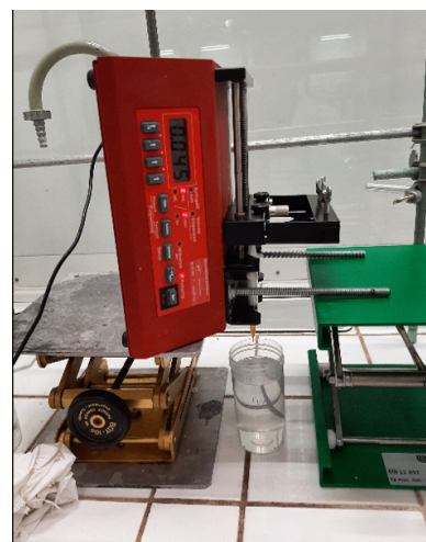
Figure 11: Vertical setup of syringe pump that is in direct contact with the coagulation bath. The coagulation bath can consist of water, ethanol or a mixture of both.
