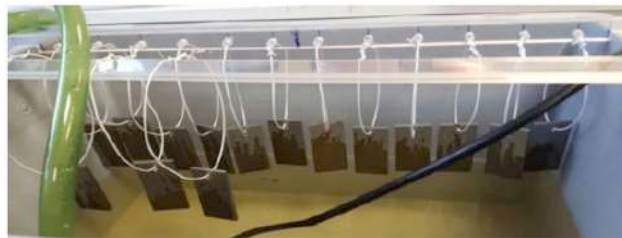
Figure .6: Coupon Testing Set-Up (Canning, 2020)
