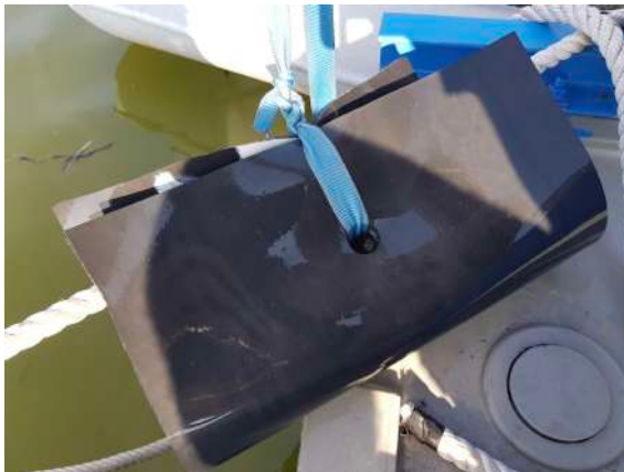
(a) The Piece of EPDM Before Submersion (b) The Piece of EPDM after Months of Exposure
