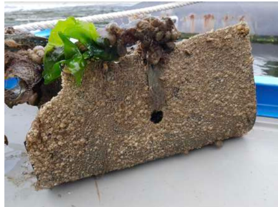
(a) The Piece of EPDM Before Submersion (b) The Piece of EPDM after Months of Exposure
