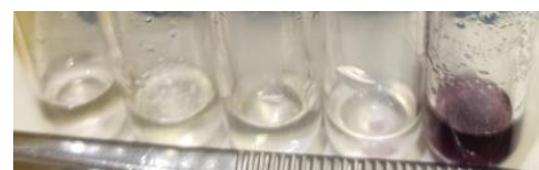
Figure 11. (From left to right) Iron chloride test of sample Roel (R), pure acetylsalicylic acid (ASA), blanco iron chloride solution (B), sample Mirjam (M) and pure salicylic acid (SA).
