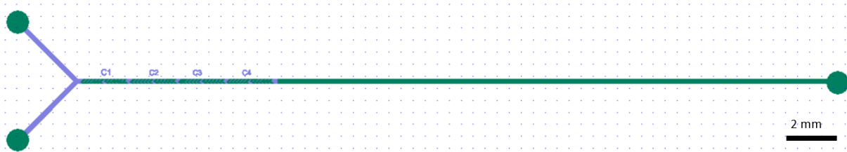
Figure 9: Design of one complete chip in CleWin3.0 with the base layer in purple and the added height structures in the second green layer.
