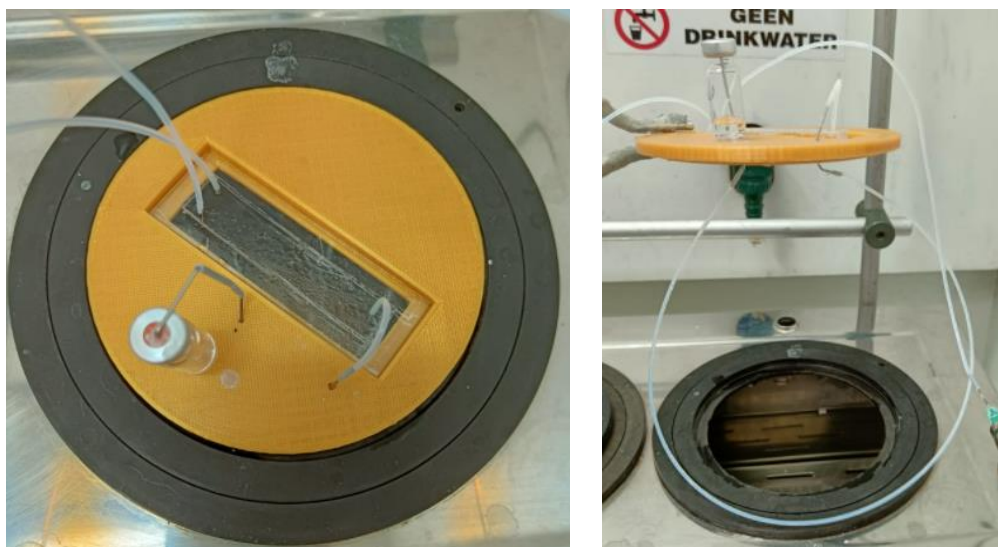
Figure 25: Prototype 3 with the proposed adjustments: on the left the capped HPLC vial with sharp needle for product collection and on the right the incubation tubing connected by needles underneath the chip holder.
