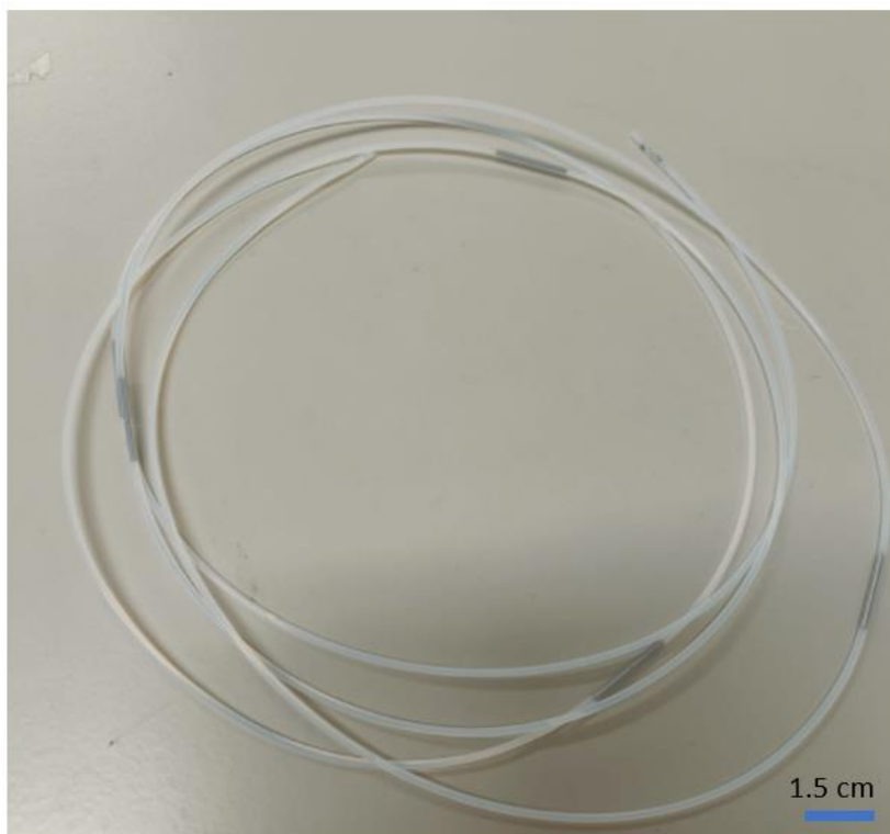
Figure 33: Incubation tubing divided into 30 cm segments representing 30 min reaction time and connected again by needles. Used to measure reaction progression in one system.
