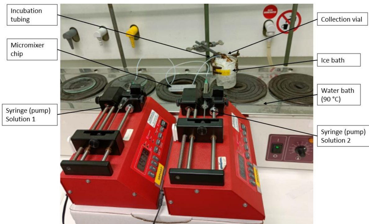
Figure 18: Prototype 1 containing 2 syringe pumps; Tubing connecting the syringes to the chip inlets; The chip on a 90 °C water bath; Incubation tubing going from the chip outlet to the collection vial on an ice bath.
