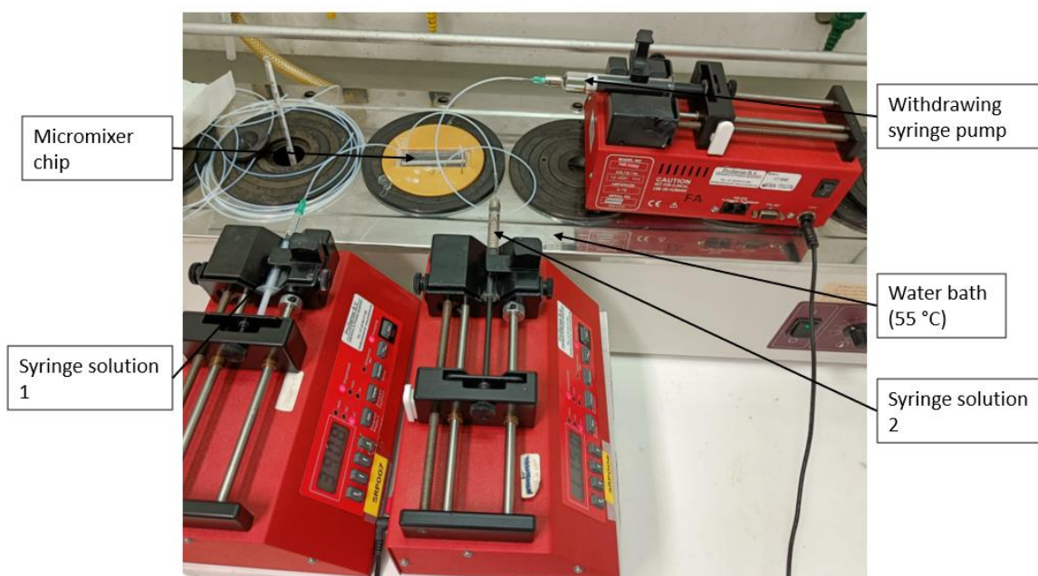
Figure 35: Addition of a third syringe pump connected to the end of the system set to withdraw at the same flowrate as the total flowrate into the system. A new syringe for solution 2 and a 10-mL syringe used for withdrawing.
