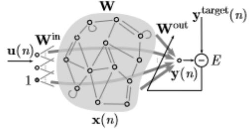
Figure 2.1: The structure of an echo state network (Lukoševičius, 2012)
