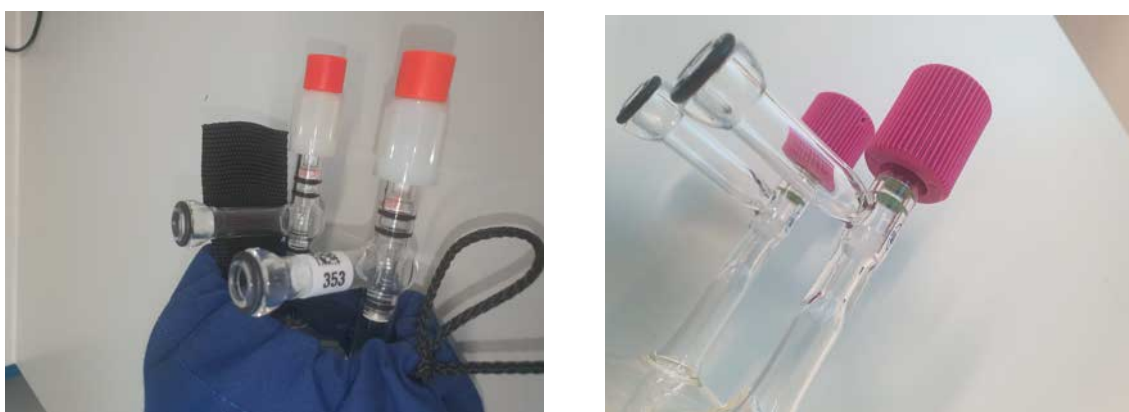
Figure 4: Figures showing the 2 types of flasks; Viton-flask on the left and PCTFE-flask on the right
