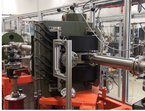
Figure 10: An overview of the 45° bending magnet. The ions enter the magnet from the right side of the image and are then bended 45° with the use of electromagnets, which are controlled at the source to steer the ions into the RFA.
