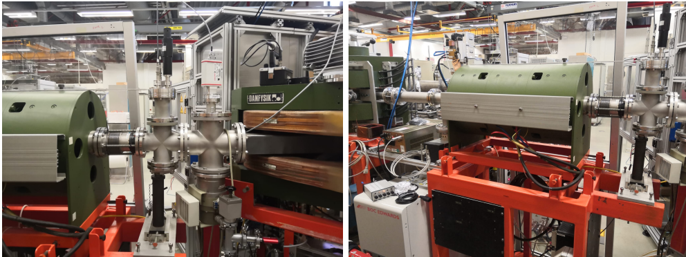
Figure 9: An overview of the first Faraday cup(left image) and the first triplet(right image). The Faraday cup can be lowered into the beamline to optimize the settings of the Ion Source, Puller and Einzel Lens before sending the ions further down the beamline. When the beam is optimized, the Faraday cup is then retracted from the beamline and the ions encounter the triplets. The triplets are then used to focus and steer the beam into the RFA at CHEOPS.
