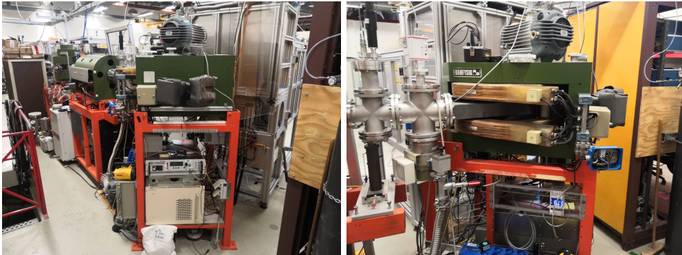
Figure 8: An overview of the 110° bending magnet. The bending magnet is used to separate the different isotopes and charge states by making use of the mass-over-charge ratio of the different ions. By measuring the ion current at the first Faraday cup and compare it to the current provided to the magnet, the different ions can be separated and then send further down the beamline.
