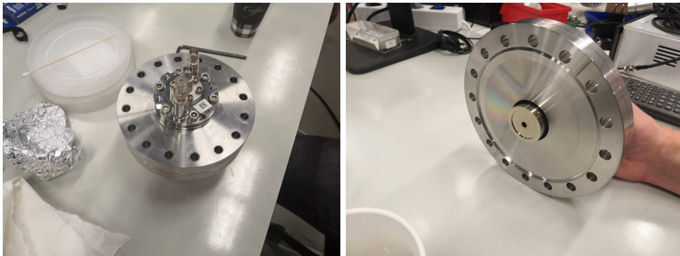
Figure 12: Left: The topside of the RFA. The inputs on top of the RFA from left to right are: The retarding grid voltage, the current readout, the suppressor grid voltage. Right: The backside of the RFA. The shield is clearly visible in the middle of the flange. The hole in the middle is where the positive ions enter the RFA.
