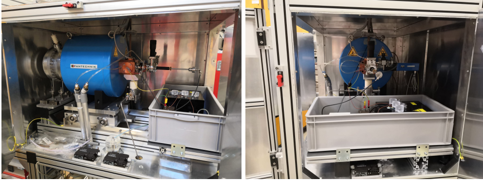
Figure 7: An overview of the ion source used in the experiments. The blue cylinder is a 1T magnet, for plasma confinement. The ions leave the magnet on the left side of the magnet (viewed from the image on the left).
