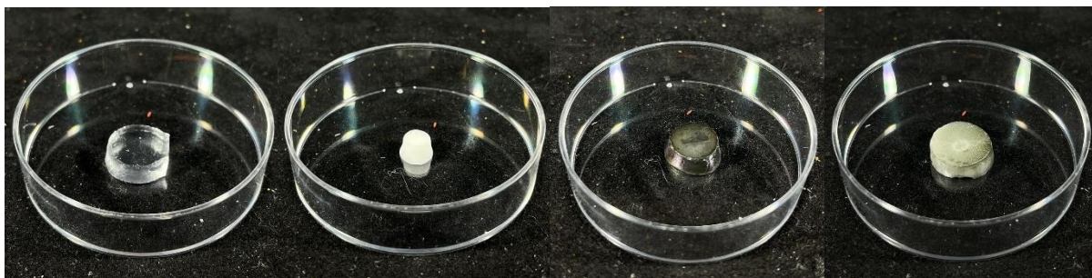
Figure 1. Pictures of double network hydrogel samples and their polypyrrole coated counterparts (from left to right): Pure PAAm (transparent), PAAm-PSS/PDADMA(10%); PAAm-PPy (transparent); PAAm-PSS/PDADMA(10%)-PPy. Other double network hydrogel samples (coated and uncoated) with different proportions of PSS/PDADMA has similar features with PAAm-PSS/PDADMA(10%)
