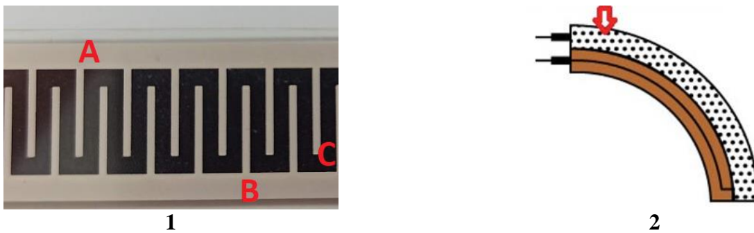
Figure 11 Close-up of resistive flex sensor (1) with flexible plates (A and B), and conductive elastomer (C). Bent flex sensor with conductive dots (red arrow) and plates (2)
