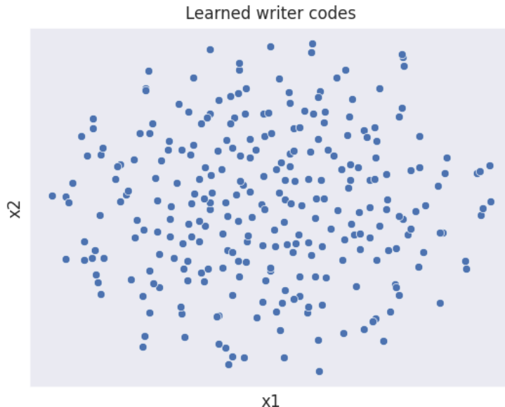
Figure 4.2: Writer codes learned through backpropagation for FPHTR-18, reduced to two dimensions using t-SNE [101]. Although it is difficult to draw hard conclusions from such a plot, the lack of meaningful style clusters seems to suggest that the writer codes are not used effectively by the model.
