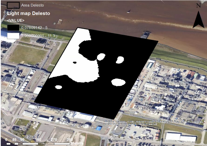
Figure 7.6: Figure which displays where there is light pollution at the Delesto factory, made in ArcGIS. In the black area the amount of lux is below 5 and the white area indicates values above 5 lux.
