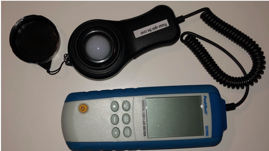
Figure 6.1: Figure which displays the PeakTech 5086, the device used to perform the lux measurements.
