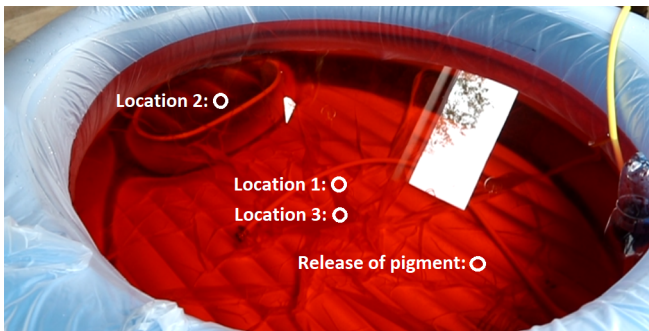
Fig. 3. This figure shows the birth pool used in the experiment and indicates at what locations the samples are taken, and where the pigment is released in the pool.
