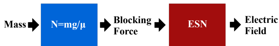
Figure 8: Gripper control pipeline. Given mass, the goal is to return an adequate electric field strength to achieve a successful lift of the cube.
