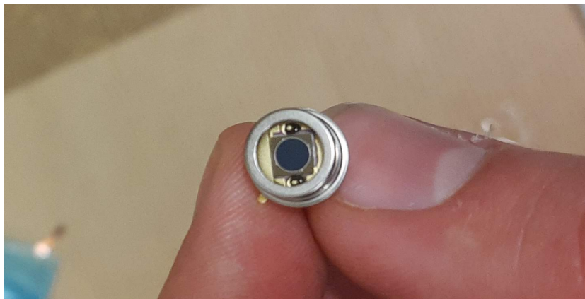
Figure 1: An avalanche photodiode. The inner black circle is the photosensitive area.
