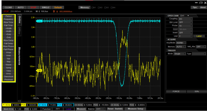
Figure 8: A trace as generated by the setup. The blue trace is from the regular photodiode, while the yellow one is from the APD. As this trace is from a test measurement, the noise in the blue trace is caused by a noisy laserdiode. During the actual measurements this was not present.
