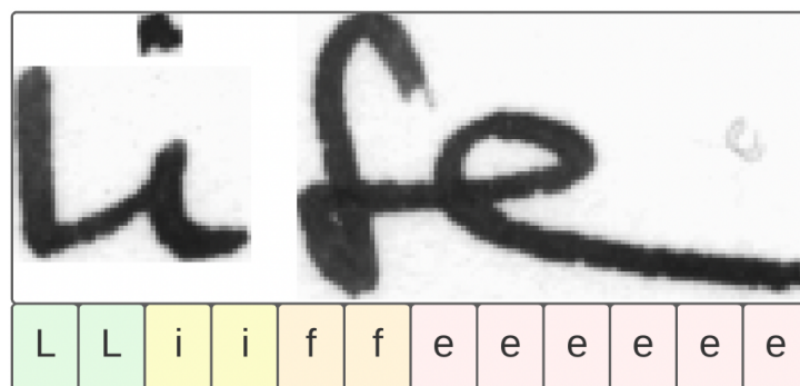
Figure 10: An example of an output that correctly matches the classifications to the location of the input characters. At each output position a token is predicted. Note how that also entails predicting parts of a character that visually do not resemble the real token — e.g. at the end of the e character.
