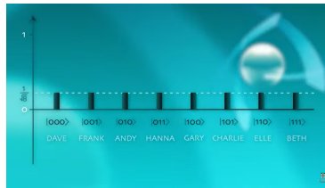
Figure 16: This is an example of Grover's algorithm for N = 8 element in the list. This is the representation of the initial wave function where each state has equal probability \frac{1}{8} to be chosen and hence the amplitude of each state is \frac{1}{\sqrt{8}} [Morello, a].
