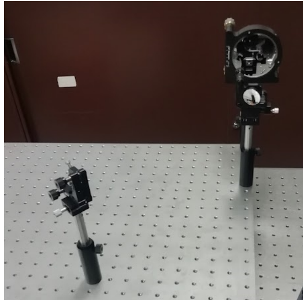
Figure 8: Alignment of the M1 mirror, with the use of 2 reference mirrors.
