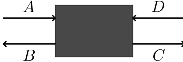
Figure 2.1: Pictorial definition of the scattering matrix \mathbf{S} : to give B and C in terms of A and D .
