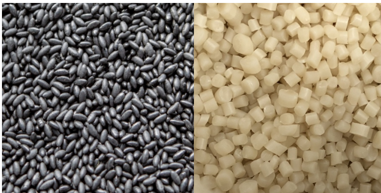
Figure 22: GreenFill granules (left) and PHA granules (right) (Biodegradable Grass Infill - GreenFill, 2022) (Zylberg, 2021).
