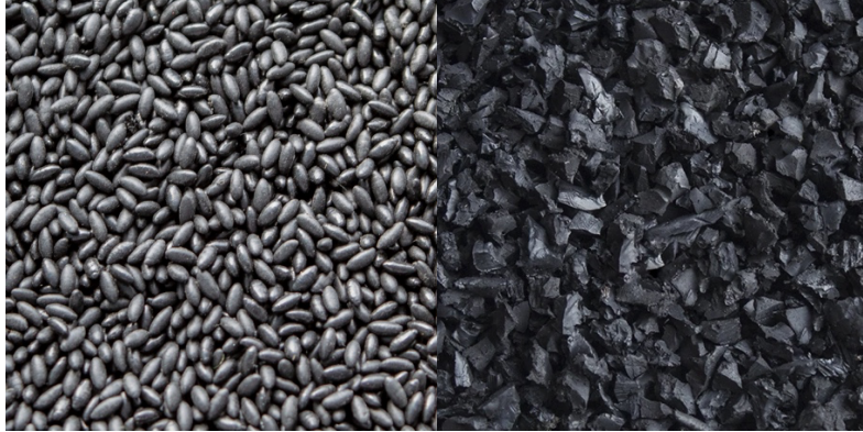
Figure 17: GreenFill granules (left) and SBR ELT granules (right) (Biodegradable Grass Infill - GreenFill, 2022) (Styrene-Butadiene Rubber | Chemical Compound, n.d.).
