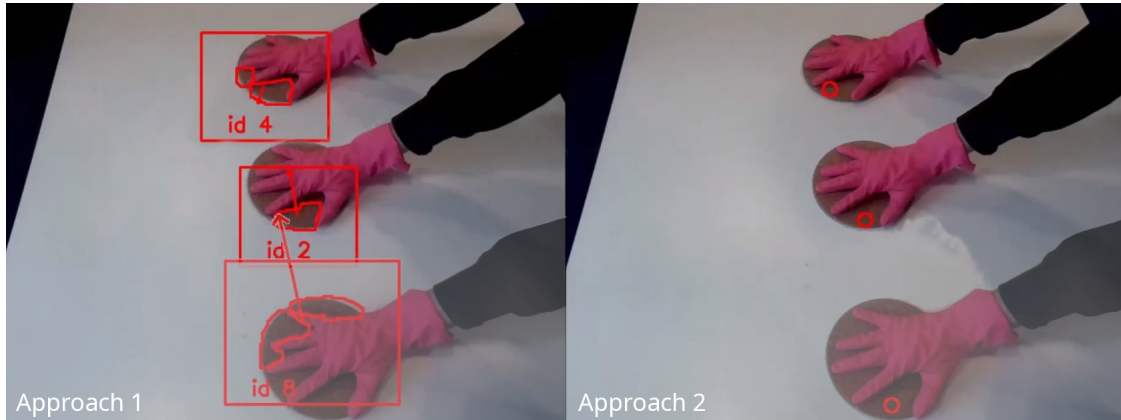
Figure 4.3: Comparing approaches 1 and 2 on a moving scenario video. Images depict hands from three different frames, as the brown coaster is being moved from the bottom of the table to the top.
