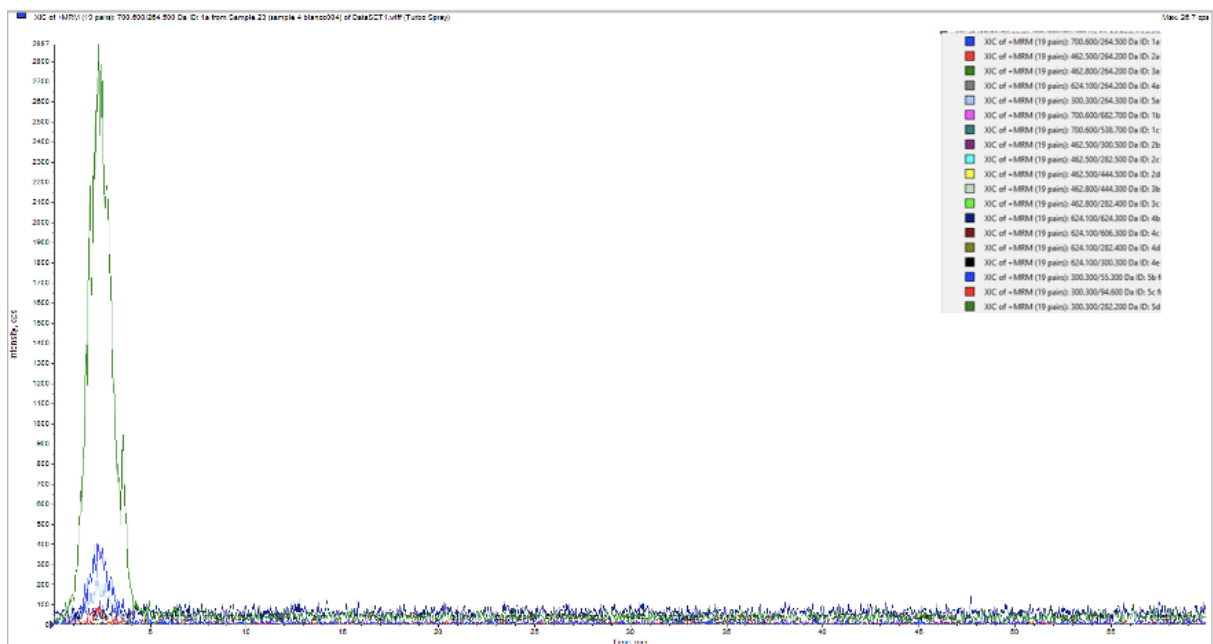
Figure 85. LC-MS/MS chromatogram blank measurement using an isocratic elution of 55% mobile phase B showing the intensity (cps) plotted against the time (min) eluting the sphingolipid standard D-sphingosine. The legend at the top right shows the colors of the product ions of the sphingolipid standards.
