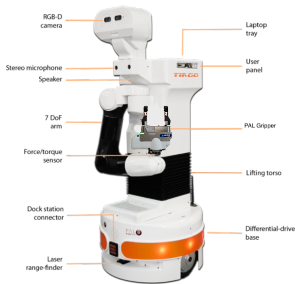
Figure 3.9: TIAGo robot from PAL Robotics, the figure describes the elements of the TIAGo robot hardware.
