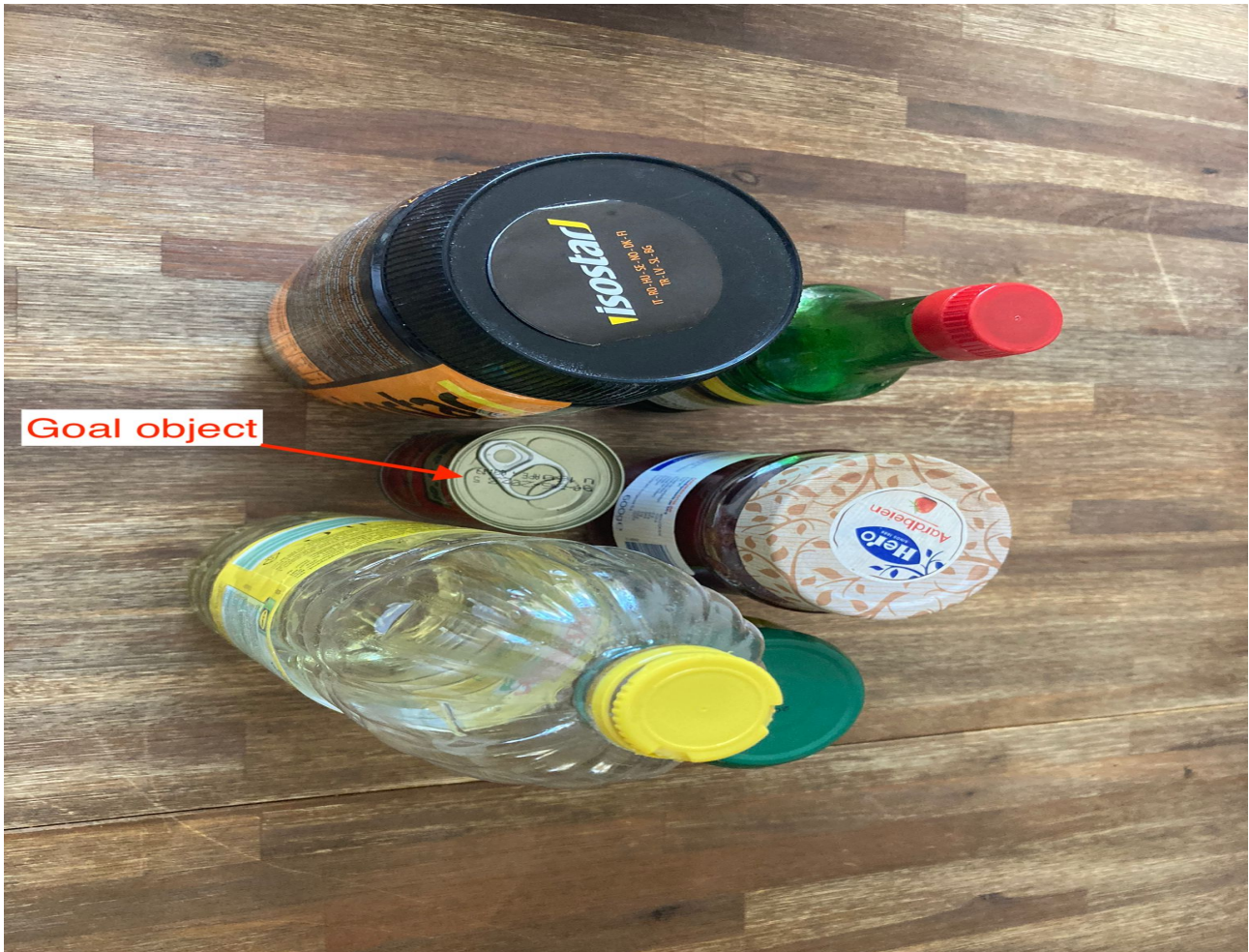
Figure 3.13: A scenario where grasping the goal object directly is impossible. An approach of grasping and removing obstacles is suitable to reach the final goal object.
