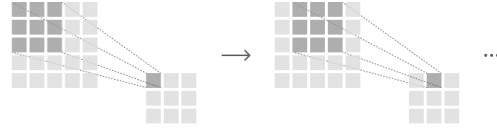
Figure B.1: A depiction of a two dimensional convolution. The dark grey area represents a 3x3 filter that slides over the pixels, computing the dot product between the overlaid area and the filter and assigning it as a pixel to the resulting image.
