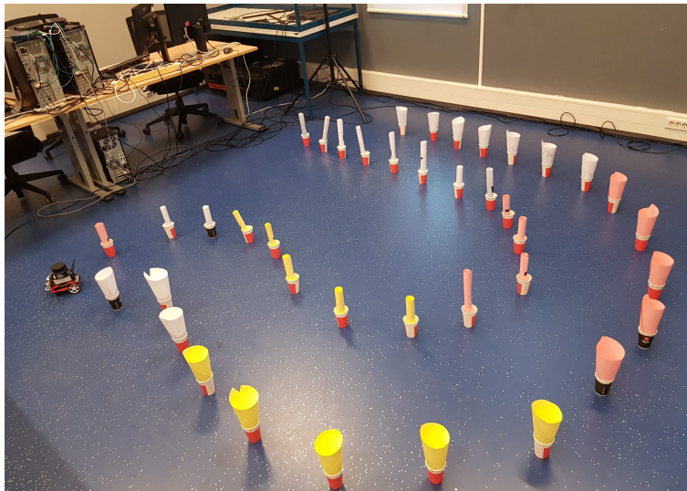
Figure 28: Photo of the real-life test track designed to test and compare the self-driving software. Due to limited space, this track was chosen in order to include at least one left turn, one right turn, and one straight region.
