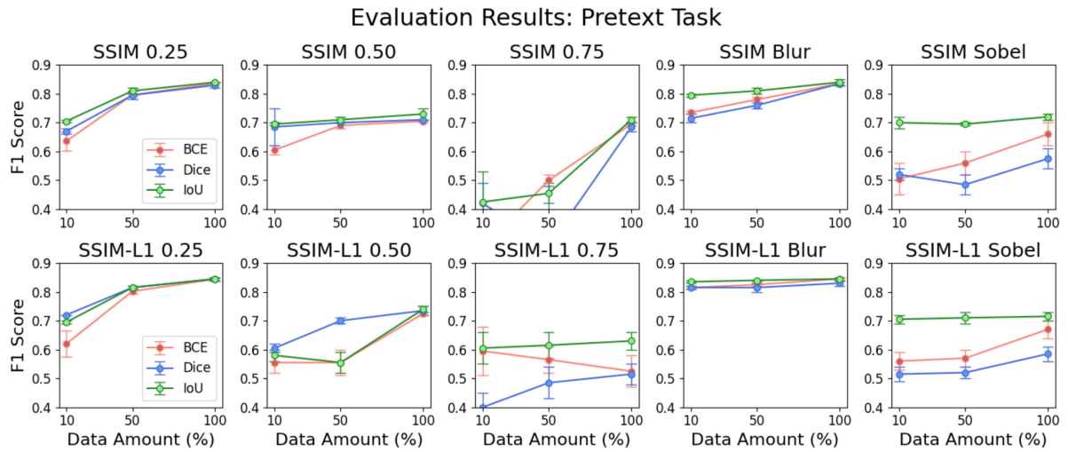
Figure 5.2: Evaluation of the self-supervised pretext task using F1-scores. The mean of the 5 folds for the BCE, Dice, and IoU loss functions were computed and is indicated by the red, blue, and green points respectively. The top row displays the scores using the SSIM loss of the pretext task, while the bottom row displays the SSIM-L1 loss.
