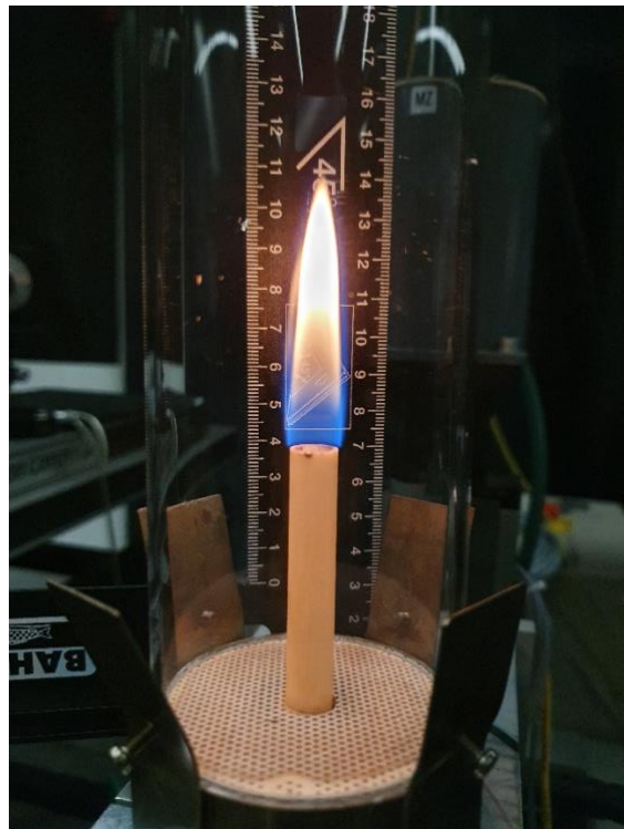
Figure 3-3. Details of diffusion burner (left) and a produced co-flow diffusion flame (right). Figure (left) adapted from A.V. Sepman et al. (2013), photo (right) from own work.
