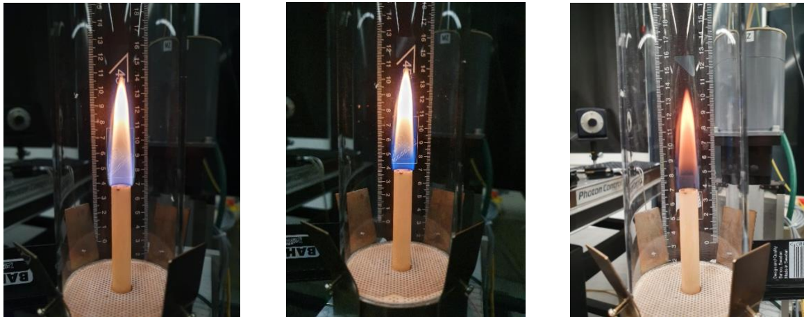
Figure 8-2. From left to right, \text{CH}_4 + \text{NH}_3 , \text{CH}_4 + \text{N}_2 , and pure \text{CH}_4 . \text{CH}_4 flow 0,25 L/min.
