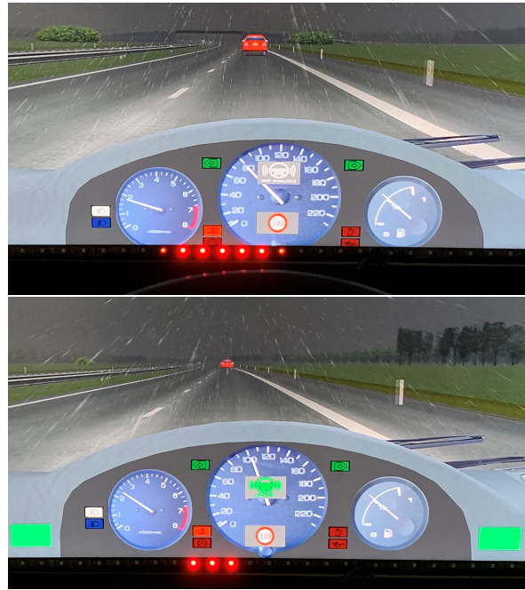
Figure 2.4: Two examples of the vehicle representation on the LED strip. The top figure shows a vehicle that is closer to the ego vehicle and the bottom figure shows a vehicle that is further away.
