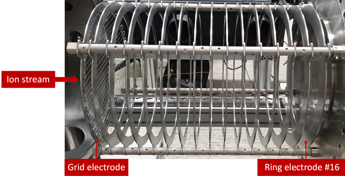
Figure 29: DC cage structure. The left ring electrode corresponds to the grid electrode or ring electrode #1. The right ring electrode corresponds to #16. In between, ring electrodes #2–#15. The ion stream is also indicated.
