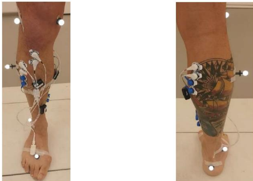
Figure 13: Image indicating the placement of the 3D CGA sensors with the optical markers and the Oro sensor system. Source: (Christian Greve et al., 2022)
