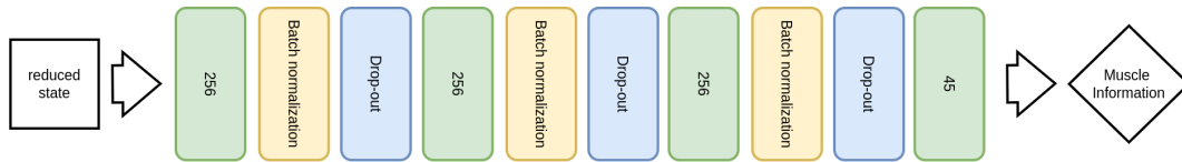
Figure 4.2: Architecture of the best performing muscle information prediction network. Green blocks represent fully-connected layers with the respective number of units displayed. Yellow blocks represent batch normalization, and blue blocks represent drop-out regularization.
