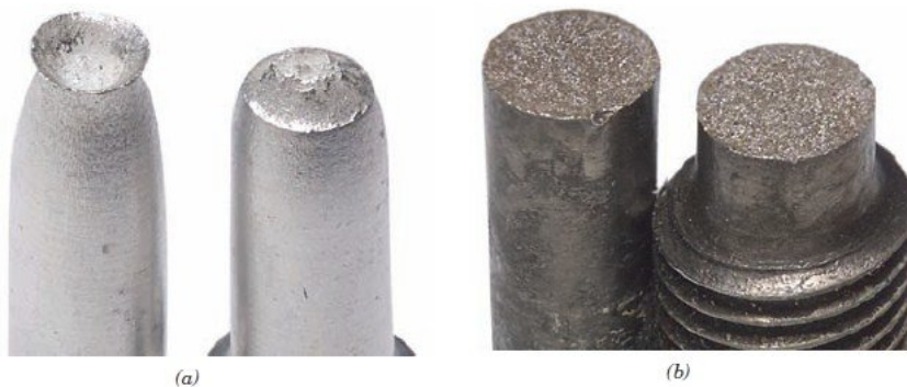
Figure 2.10: (a) Ductile cup-and-cone fracture in aluminium and (b) brittle fracture in mild steel [24].
