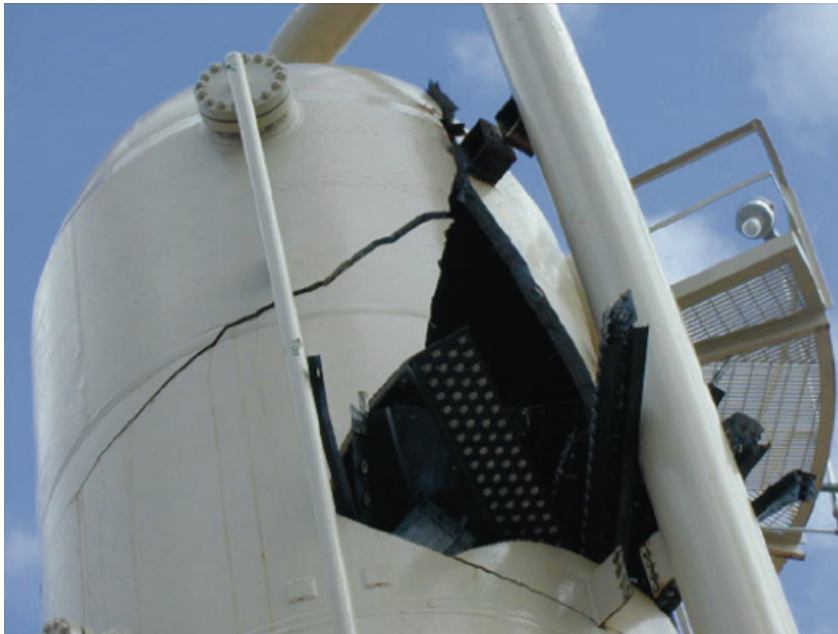
Figure 1.1: Brittle fracture of a pressure vessel [1].
