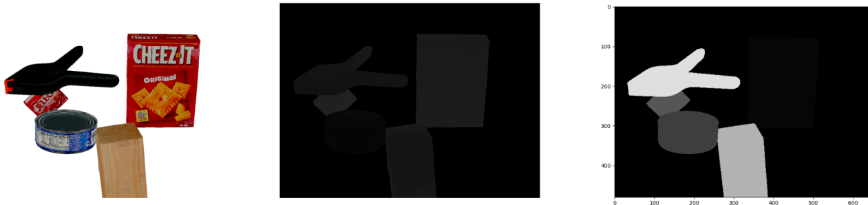
Figure 4.2: YCB-Video: Sample RGB image with corresponding depth image and label mask. (L-R: large_clamp, gelatin_box, tuna_fish_can, wood_block, cracker_box)
