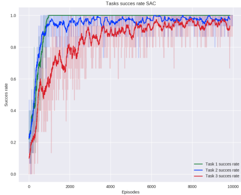
Figure 4.5: Success rate of all three tasks using the Soft Actor-Critic algorithm. Green is the first task, blue the second task, and red the third task.
