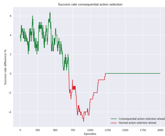
Figure D.2: Success rate difference of traditional SAC versus consequential action-selection (definition 2).
