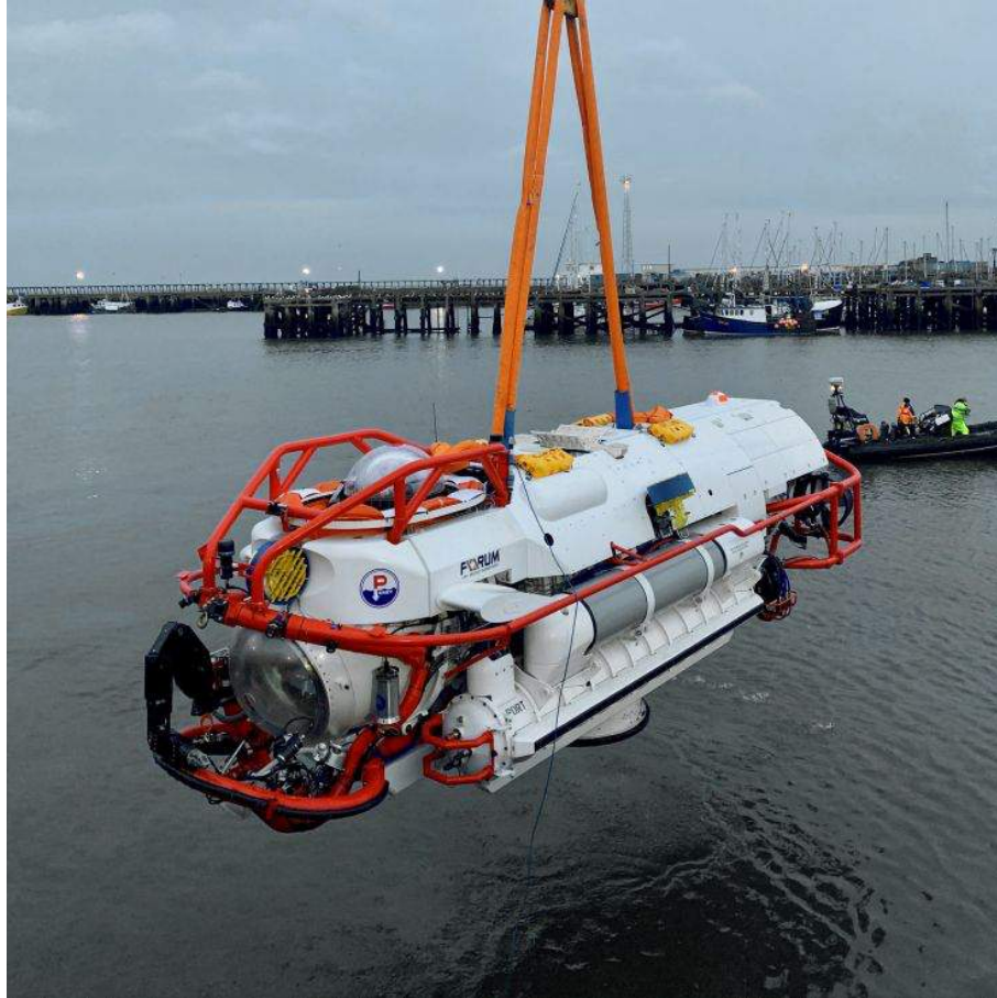
Figure 2.1: The LR11, one of the newest submarine rescue vehicles (Richard S., 2021)
