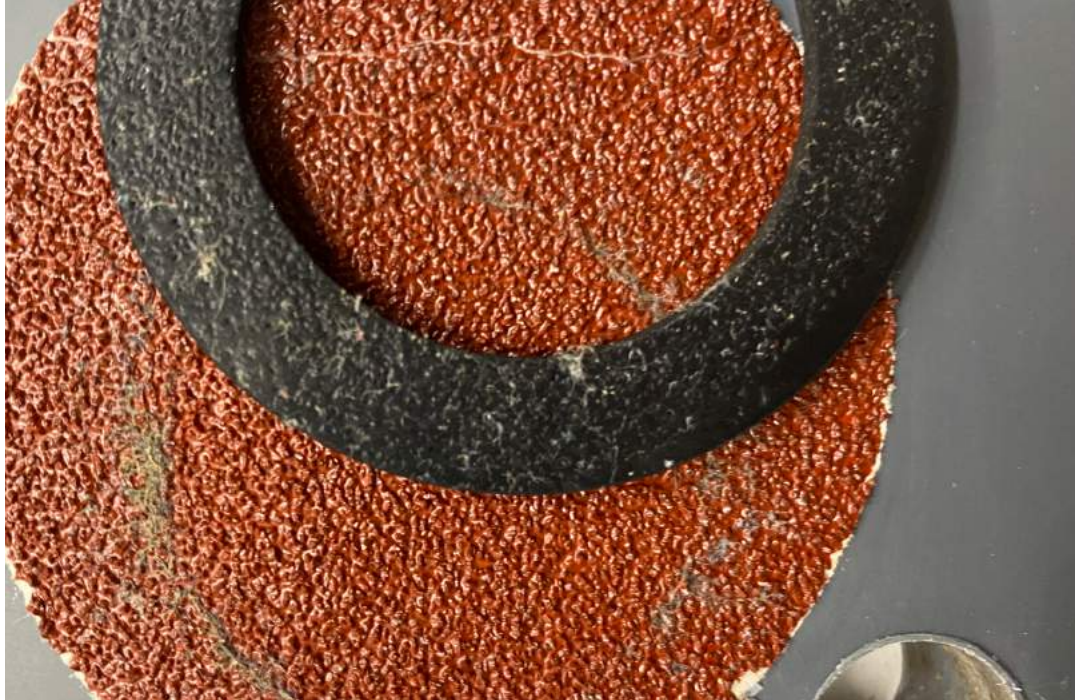
Figure 6.16: Contamination of the sandpaper and seal after a set of experiments.
