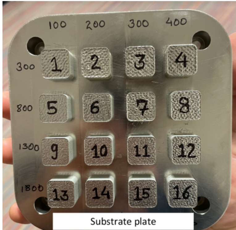
Figure 8. Substrate plate with 16 samples manufactured at different laser powers and scanning speeds.
