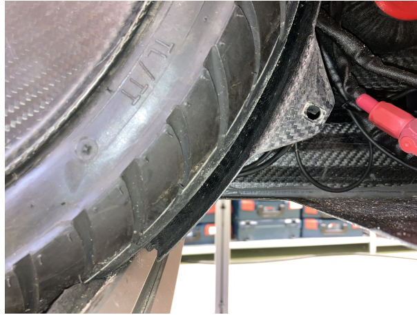
Figure 3.2: The wheel shell that is located around a majority of the wheel. This relatively complicated part will not be simulated.
