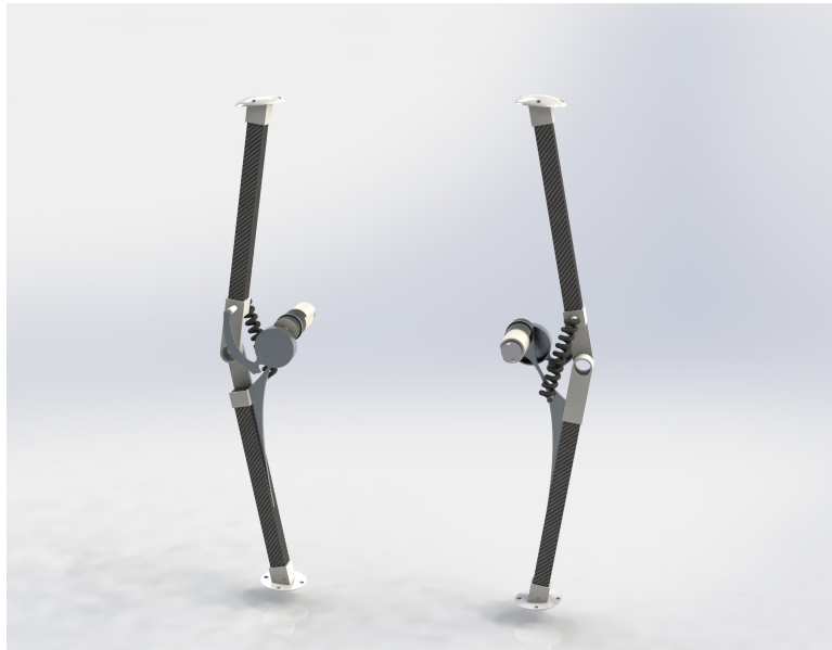
Figure 6.2: Rendering from Solidworks of two parallel legs, with a linear spring used at the joint of the legs.
