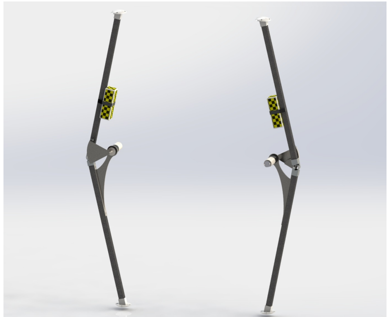
Figure 1.2: CAD model of two parallel bars. The cam is the triangular shaped object which is actuated by the circular white motor, which also contains a small gearbox. The torsion spring is embedded in the joint.
