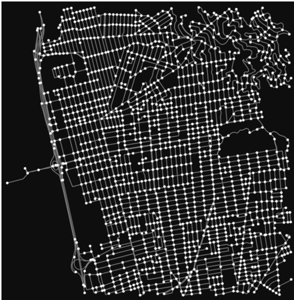
Figure 3.1 Simplified OSM graph of Berkeley obtained using OSMnx, the graph has 1449 nodes and 4957 edges.
