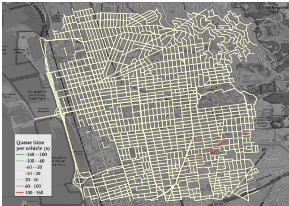
Figure C.4 Queue difference for all links in the traffic network of scenario 3 versus the base case without charging expressed as (average) queue time for all vehicles that traverse over that link.
