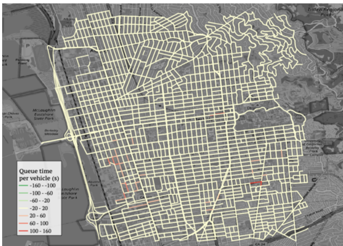
Figure 9.1 Queue difference for all links in the traffic network of scenario 1 versus the base case without charging expressed as (average) queue time for all vehicles that traverse over that link. Agents reroute every 2 minutes.
