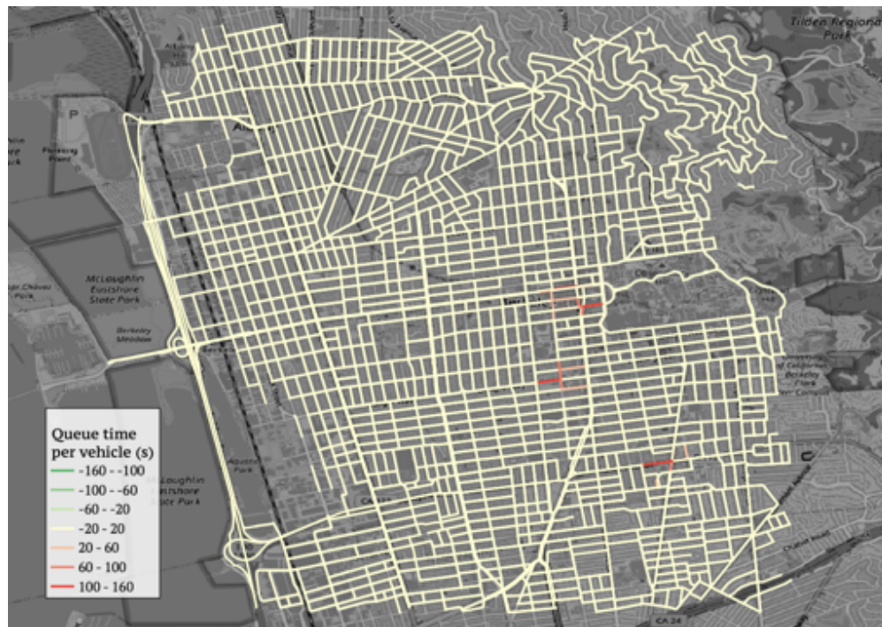
Figure C.3 Queue difference for all links in the traffic network of scenario 2 versus the base case without charging expressed as (average) queue time for all vehicles that traverse over that link.
