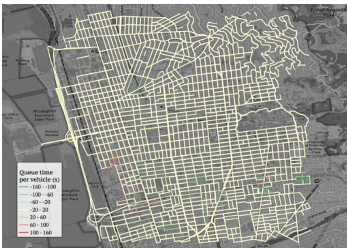
Figure 9.3 Queue difference for all links in the traffic network of scenario 1 with rerouting versus the scenario 1 without rerouting expressed as (average) queue time for all vehicles that traverse over that link.
