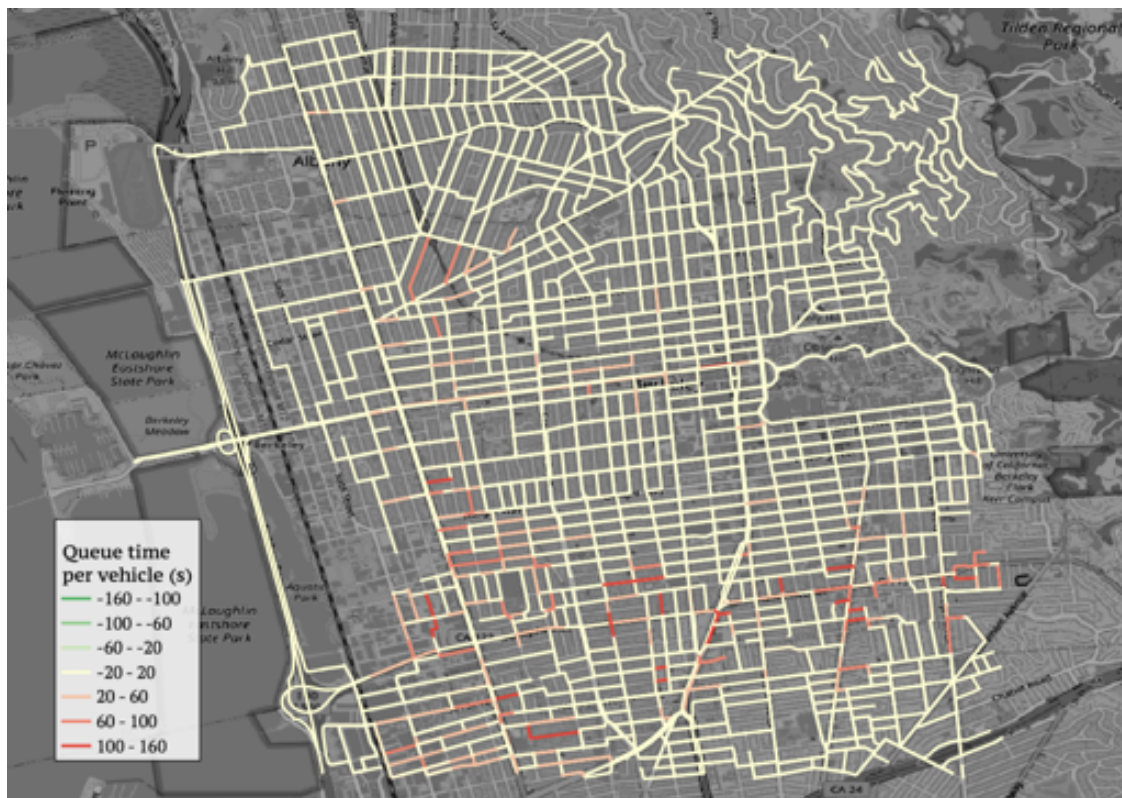
Figure 9.2 Queue difference for all links in the traffic network of scenario 1 versus the base case without charging expressed as (average) queue time for all vehicles that traverse over that link. Agents do not revise their route.
