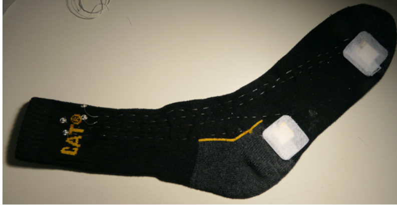
Figure 17: Picture of final fabricated sock with buttons as connectors and padding on the sensors
