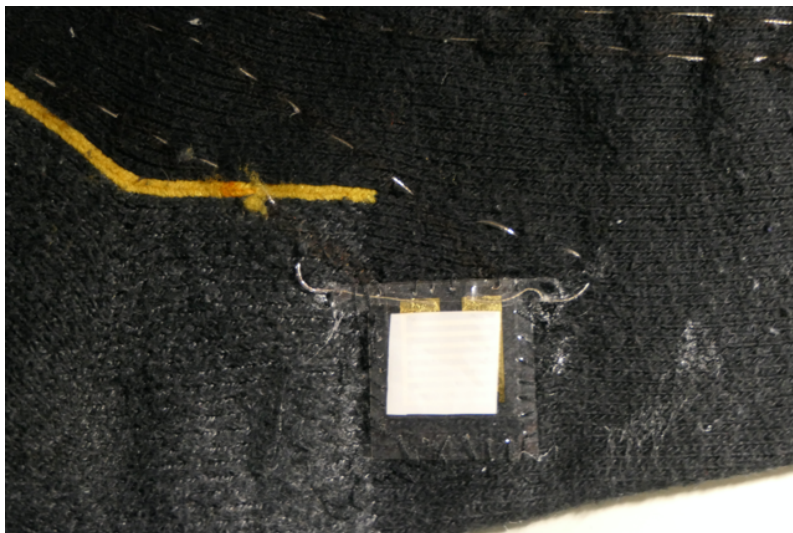
Figure 26: Picture of a sensor with interdigitated electrodes and conductive yarn wires mounted on a sock
