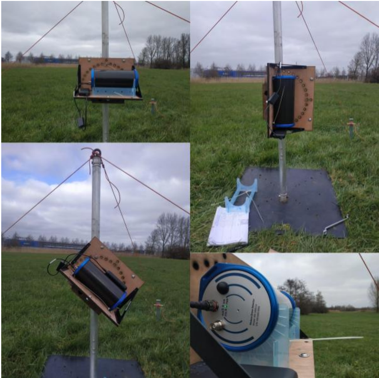
Figure 5.6: Photographs of the experimental setup that was used to measure with the split detector at various angles. The side where the cable comes out of the detector is the front. The crystals are positioned to the back of the detector (as illustrated in Figure 4.1).
