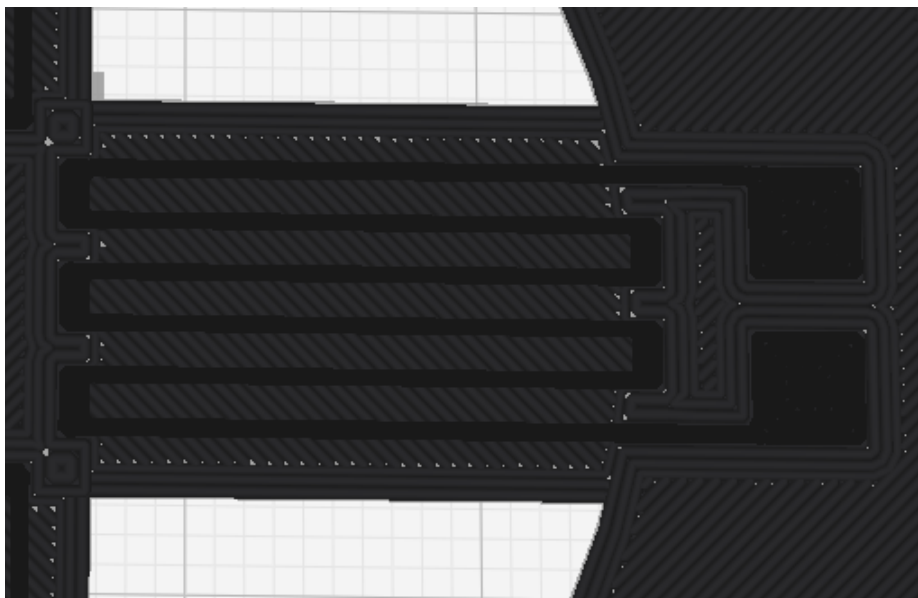
Figure A1: Example of integration of two separate bodies in the slicer
