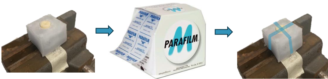
Figure 3 The two plugs are placed on top of each other, and a sponge cube surrounds them. Parafilm strips keep the whole structure together. Thin blue lines represent the PARAFILM strips
