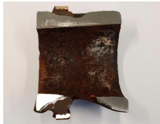
Figure 17 Thickwalled munition with leakpaths due to galvanic corrosion of the driving bands
