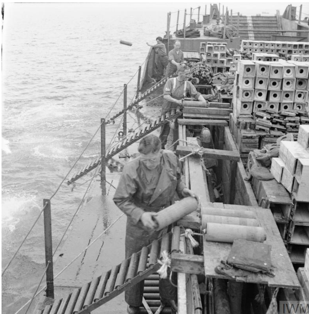
On arrival at the ammunition dumping ground off Cairnryan, near Stranraer, Wigtonshire, Scotland, members of the Royal Army Ordnance Corps (RAOC) place shells on gravity rollers that take the ammunition over the side of the ship and into the sea. Note the man in the background who is simply throwing ammunition overboard. (source: IWM, H 42208)
