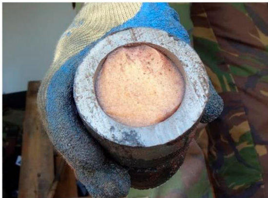
Figure 17 Thickwalled munition with leakpaths due to galvanic corrosion of the driving bands
