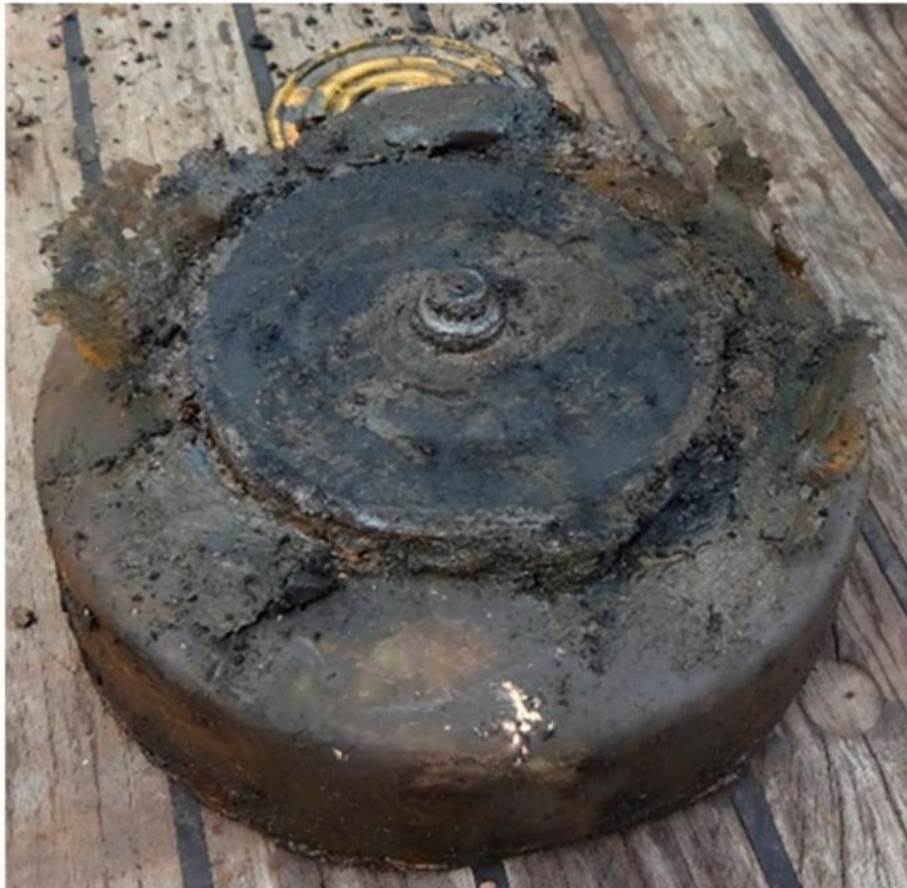
Figure 16. An almost completely corroded landmine
