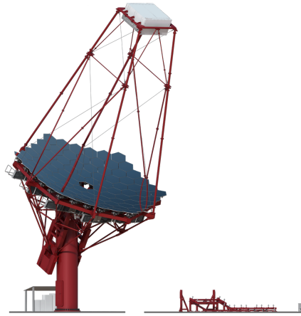
Figure 4: The design of the Medium-Sized Telescope [22]
