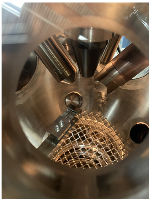
Figure 3.2: Image of the heart of the measurement chamber. From left to right a helium lamp, the entrance to the electron energy analyzer, and the X-ray source can be seen.
